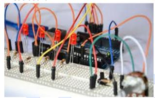
Breadboards are perfect for prototyping. When you first design your circuit, a breadboard allows you to quickly build, test, and change your connections. Breadboard wires (4A max) come pre-assembled with either a male or female connector on each end, and are compatible with header pins and DuPont connectors. We also offer solid core wire sets for breadboards, which are a bit less of an eyesore.
