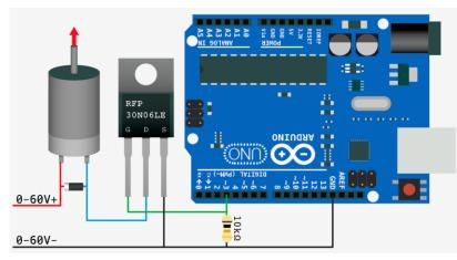
The 10k resistor is used to pull the circuit to ground when there is no signal from the Arduino (use a resistor value greater than or equal to 10k). When using a MOSFET with a motor or other inductor, make sure to use a flyback diode to protect the MOSFET from current surges.
