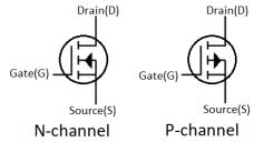
While MOSFETS work best as on/off switches, they do have a limited range where they can constrict current. This occurs when  $V_{gate} \sim V_{source} - V_{threshold}$  (P type) or  $V_{gate} \sim V_{source} + V_{threshold}$  (N type).
