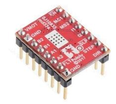
To use this motor driver, you will need a stepper motor, a DC power supply, and a PWM signal. If you are using a microcontroller (or Arduino), recognize that neither of these can supply enough current to run a stepper motor, and you will need an additional power source.
